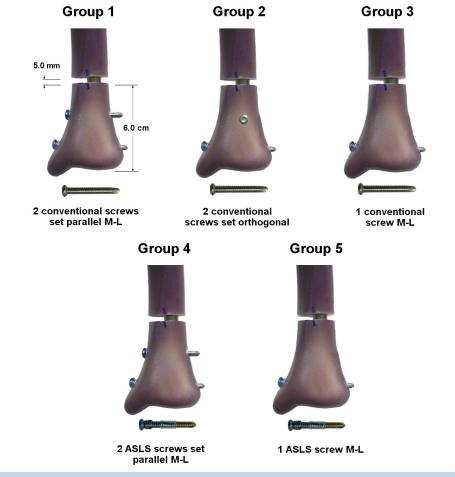
**Figure 2.** The five distinct distal locking configurations tested in this study with the type of screw employed for each.
