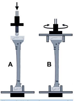
**Figure 3.** Mechanical testing setup for axial compression (**A**) and torsional (**B**) testing.
