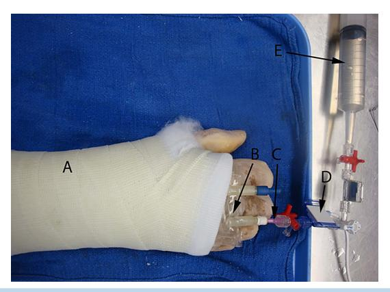
**Figure 2.** Test set up for pressure measurements. **A**. fiberglass cast, **B**. saline bag under the short-arm cast, **C**. 15 gauge needle, **D**. pressure transducer, **E**. 60 mL syringe.
